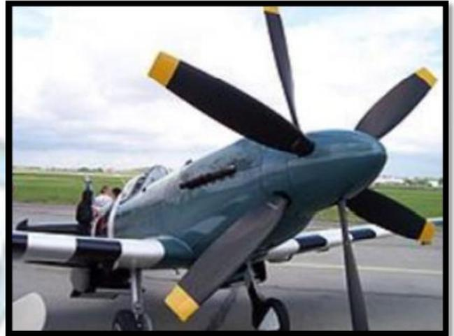
Contra Rotating Propellers by default are usually extremely noisy hence do not suit the application of passenger carriage due to EPA regulations. Commercial carriers have trialled their usage in the past due to promised efficiency gains but stopped short due to noise restriction problems.
