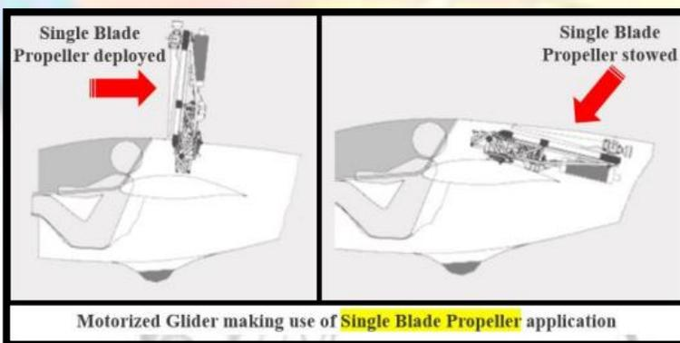
It also creates less drag when that single blade is stowed in-line with the engine mast.
